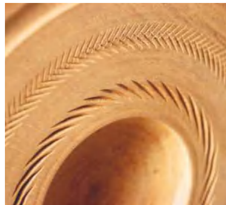
▲ Deeper profiles are well defined if they aren't too close to each other
